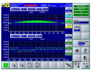
Utilizing intelligent sensor and scanner techniques, the Mahlo QMS systems measure on-line continuously and with extreme precision and speed. The computer interface is Windows Embedded based and is fully open and conforms to all industrial communications standards. Ease of use and configurability were built in from the ground up and the menus and functions are very easy to understand with a short learning curve.
