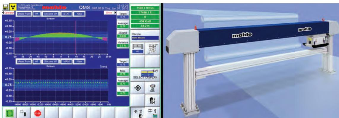
FIGURE 1. Typical on-line web-gauging system
